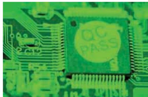
*An X-ray inspection may be the final step before "passing" an IC.*
